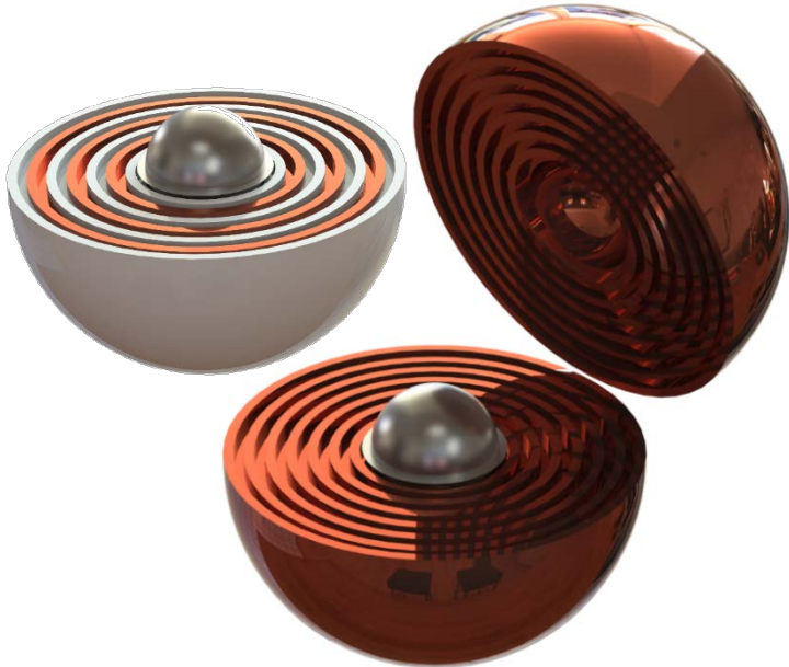
Fig. 2. Preliminary Solidworks® Computer-Aided Design (CAD) rendering of the SCRαP integral experiment. The BeRP ball can be seen in the center of the nested Cu ( bottom ) and Cu/polyethylene ( top ) shells.
