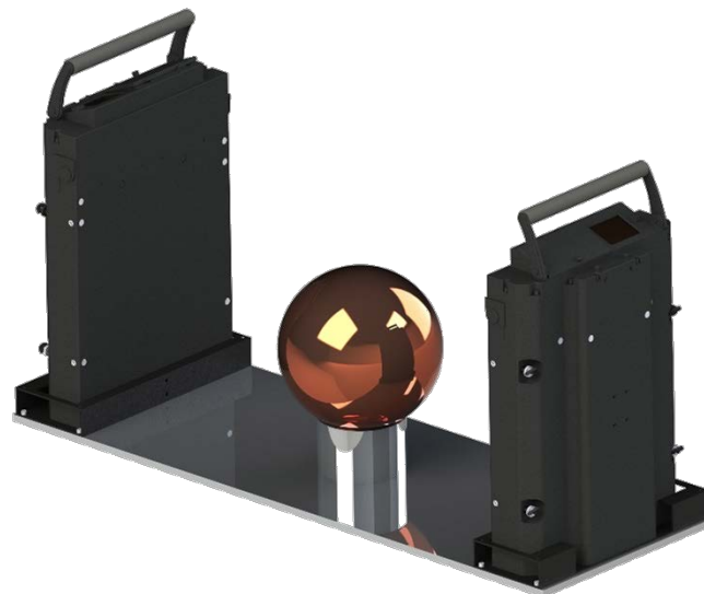
Fig. 1. Preliminary Solidworks® Computer-Aided Design (CAD) rendering of the SCR \alpha P integral experiment. The BeRP ball inside nested Cu is in the center. Two MC15 detector systems are used to estimate the multiplication of each configuration.
