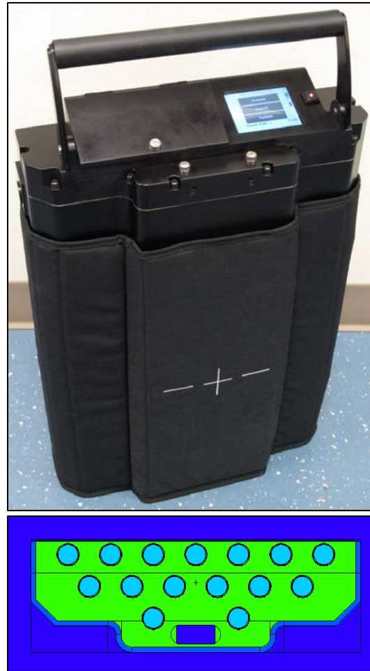
Fig. 4. Photograph and MCNP® model of the MC15 detector system.
