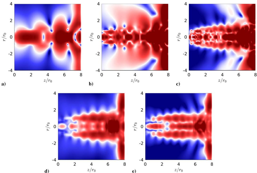
**Fig. 15** Pressure levels for the axisymmetric mode for  $M = 1$  at the frequencies of a) the dominant tone at  $St = 0.31$ , of its b) first and c) second harmonics and of d) the first and e) second non-harmonic peaks. The color scales range from a) 160 to 190 dB/St, b) 140 to 170 dB/St and (c–e) 130 to 160 dB/St, from blue to red.
