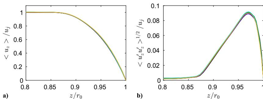
Fig. 1 Nozzle-exit radial profiles of a) mean axial velocity  $\langle u_z \rangle / u_j$  and b) axial turbulence intensity  $\langle u'_z u'_z \rangle^{1/2} / u_j$ ; —  $M = 0.6$ ; —  $M = 0.75$ ; —  $M = 0.8$ ; —  $M = 0.9$ ; —  $M = 1$ ; —  $M = 1.1$ ; —  $M = 1.3$ .
