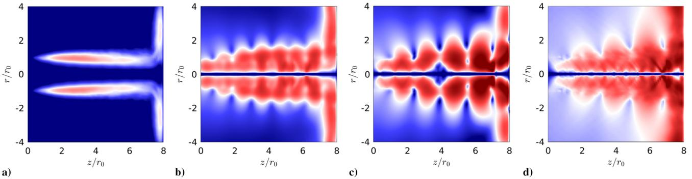
**Fig. 14** Pressure levels for the first helical mode at the peak frequencies a)  $St = 1.16$  for  $M = 0.6$ , b)  $St = 0.7$  for  $M = 0.9$ , c)  $St = 0.46$  for  $M = 1.1$  and d)  $St = 0.34$  for  $M = 1.3$ . The color scales range from a) 130 to 160 dB/St, b) 130 to 170 dB/St, c) 150 to 180 dB/St and d) 150 to 200 dB/St, from blue to red.
