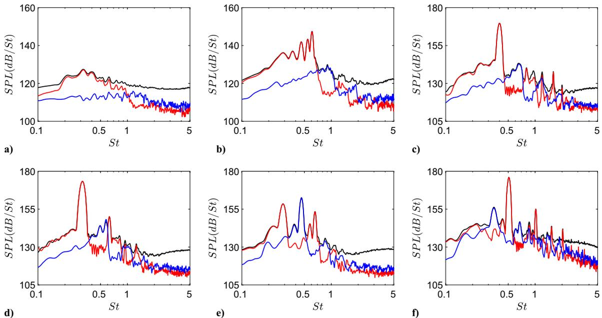
**Fig. 6 Sound pressure levels (SPL) at  $r = 1.5r_0$  and  $z = 0$  for a)  $M = 0.6$ , b)  $M = 0.75$ , c)  $M = 0.9$ , d)  $M = 1$ , e)  $M = 1.1$  and f)  $M = 1.3$ : — full signal; —  $n_\theta = 0$ ; —  $n_\theta = 1$ .**
