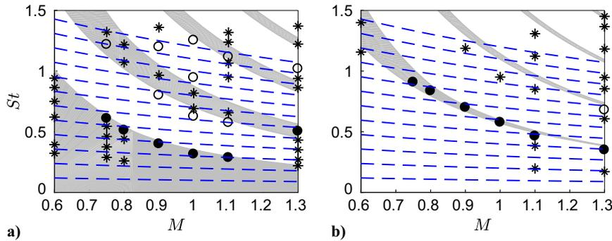
**Fig. 8** Mach number variations of the Strouhal numbers of the peaks in the near-nozzle pressure spectra for a)  $n_\theta = 0$  and b)  $n_\theta = 1$ : • and ◦ dominant tones and their harmonics; \* other peaks; (gray shading) allowable frequency bands of the free-stream upstream-propagating guided jet waves for a vortex-sheet model; - - Eq. (1) with  $N$  varying from 1 to 12.
