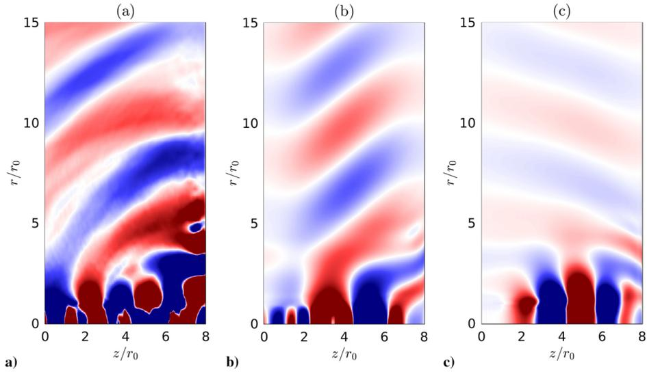
Fig. 17 Snapshots of a) the pressure fluctuations obtained by LES and the components with b) negative and c) positive wavenumbers for the jet at  $M = 0.9$  for  $n_\theta = 0$ . The color scale ranges from  $-1000$  to  $1000$  Pa, from blue to red.
