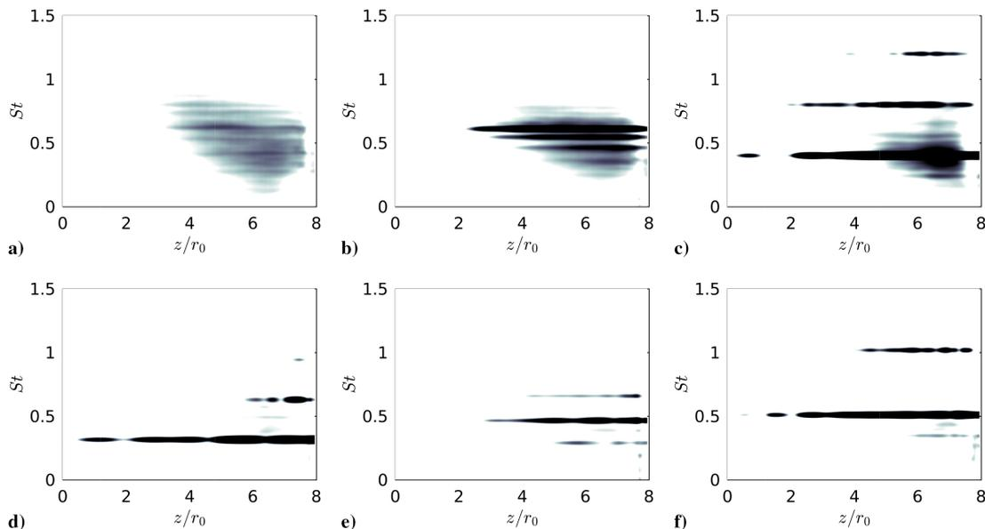
Fig. 10 Power spectral densities of the fluctuations of radial velocity  $u'_r$  normalized by the jet velocity  $u_j$  at  $r = r_0$  between the nozzle and the plate for a)  $M = 0.6$ , b)  $M = 0.75$ , c)  $M = 0.9$ , d)  $M = 1$ , e)  $M = 1.1$  and f)  $M = 1.3$ . The color scale is the same in all cases and spreads over 3 dB, from white to black.
