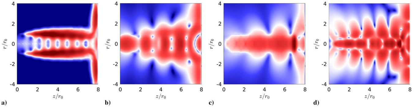
**Fig. 13** Pressure levels for the axisymmetric mode at the peak frequencies a)  $St = 0.94$  for  $M = 0.6$ , b)  $St = 0.40$  for  $M = 0.9$ , c)  $St = 0.29$  for  $M = 1.1$  and d)  $St = 0.51$  for  $M = 1.3$ . The color scales range from a) 125 to 150 dB/St, b) 150 to 200 dB/St, c) 140 to 190 dB/St and d) 150 to 200 dB/St, from blue to red.
