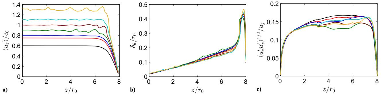
**Fig. 4** Variations of a) the centerline mean axial velocity  $\langle u_z \rangle / c_0$ , b) the shear-layer momentum thickness  $\delta_\theta / r_0$  and c) the axial turbulent intensity  $\langle u'_z u'_z \rangle^{1/2} / u_j$  at  $r = r_0$  for —  $M = 0.6$ , —  $M = 0.75$ , —  $M = 0.8$ , —  $M = 0.9$ , —  $M = 1$ , —  $M = 1.1$  and —  $M = 1.3$ .
