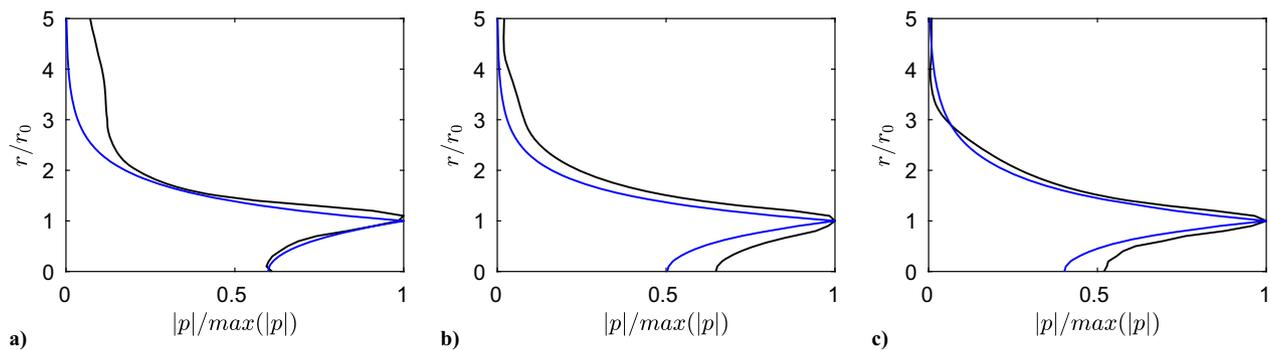
Fig. 19 — Radial profiles of rms pressure for the components with  $k > 0$  from the LES and — pressure eigenfunctions of the Kelvin-Helmholtz waves given by a vortex-sheet model [55] at the dominant tone frequency for  $n_\theta = 0$  and for a)  $M = 0.6$ , b)  $M = 0.9$  and c)  $M = 1.3$ .
