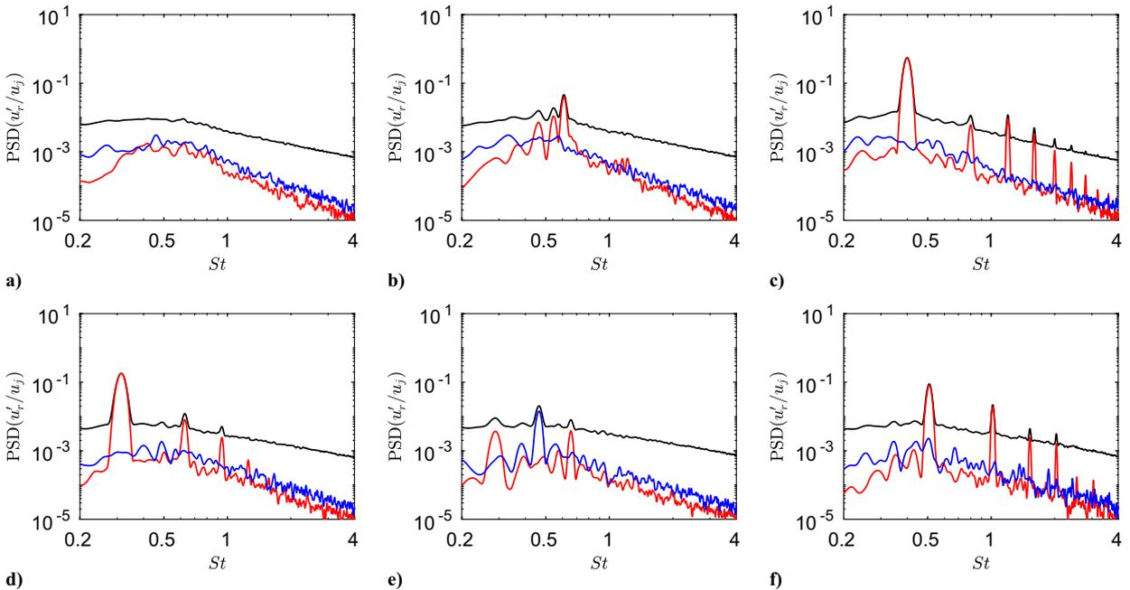
**Fig. 12** Power spectral densities of the fluctuations of radial velocity  $u'_r$  at  $r = r_0$  and  $z = 7r_0$  for a)  $M = 0.6$ , b)  $M = 0.75$ , c)  $M = 0.9$ , d)  $M = 1$ , e)  $M = 1.1$  and f)  $M = 1.3$ : — full signal; —  $n_\theta = 0$ ; —  $n_\theta = 1$ .
