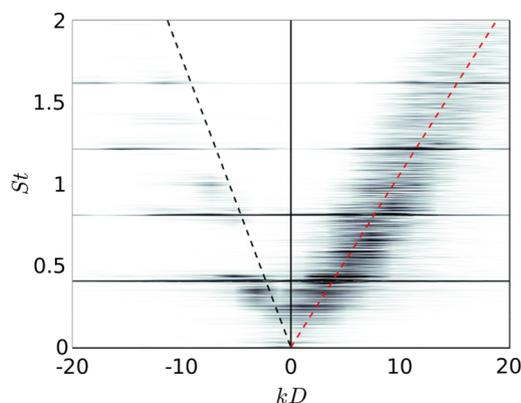
**Fig. 16** Frequency–wavenumber spectrum of the pressure fluctuations at  $r = r_0$  for the jet at  $M = 0.9$  for  $n_\theta = 0$ : ---  $k = \omega/u_c$  with  $u_c = (2/3)u_j$ ; - - -  $k = -\omega/c_0$ . The grayscale levels spread over 12 dB.
