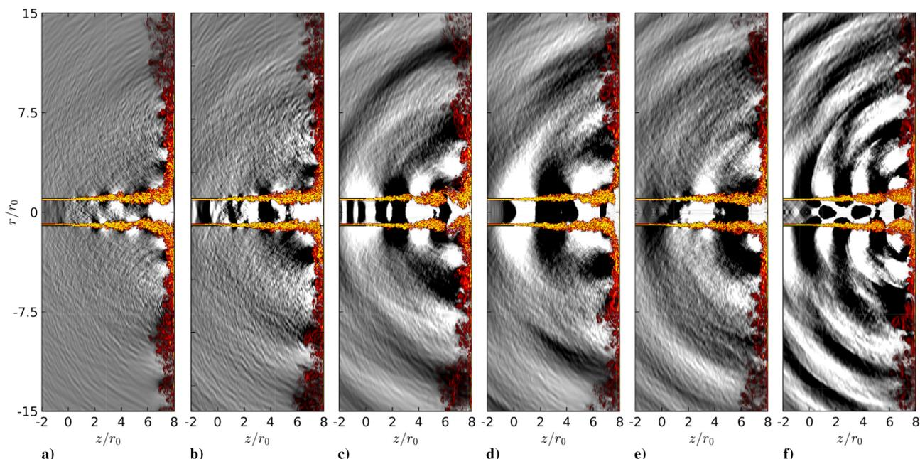
Fig. 3 Snapshots of vorticity norm in the flow and of pressure fluctuations outside in the  $(z, r)$  plane for a)  $M = 0.6$ , b)  $M = 0.75$ , c)  $M = 0.9$ , d)  $M = 1$ , e)  $M = 1.1$  and f)  $M = 1.3$ . The color scales range from 0 to  $15u_j/r_0$  for vorticity, from black to yellow, and between  $\pm 0.005p_0$  (a–c) and  $\pm 0.01p_0$  (d–f) for pressure, from black to white.
