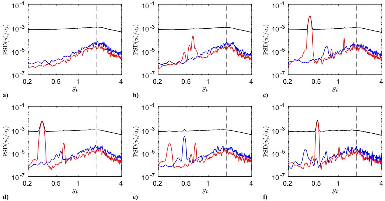
**Fig. 11** Power spectral densities of the fluctuations of radial velocity  $u'_r$  at  $r = r_0$  and  $z = 0.4r_0$  for a)  $M = 0.6$ , b)  $M = 0.75$ , c)  $M = 0.9$ , d)  $M = 1$ , e)  $M = 1.1$  and f)  $M = 1.3$ : — full signal; —  $n_\theta = 0$ ; —  $n_\theta = 1$ ; ---,  $St_0 = f\delta_0/u_j = 0.016$ .
