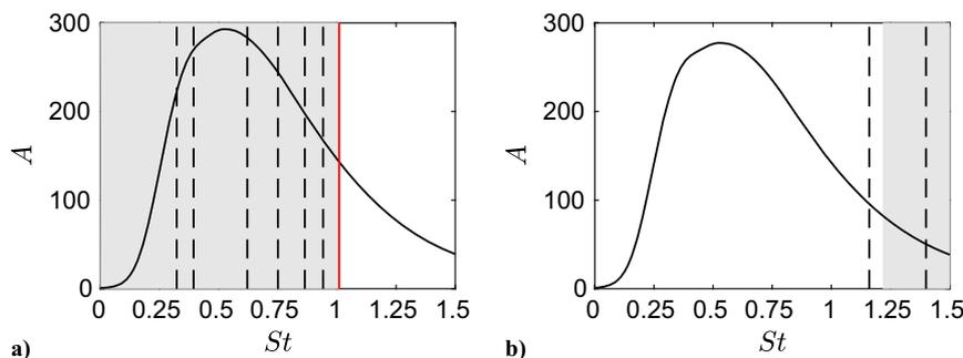
**Fig. 22** Power gain of the Kelvin–Helmholtz waves between  $z = 0$  and  $8r_0$  as a function of the Strouhal number for  $M = 0.6$  and a)  $n_\theta = 0$  and b)  $n_\theta = 1$ , - - - frequencies of the weak peaks in the near-nozzle pressure spectrum; — frequency of the least-dispersed waves; (light-gray shading) allowable frequency bands of the free-stream upstream-propagating guided jet waves.
