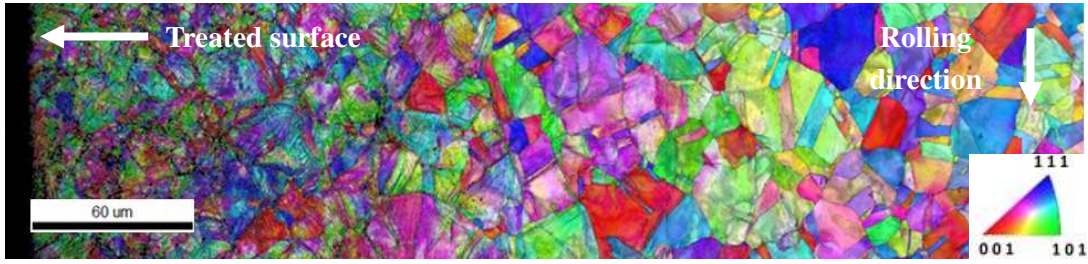
Fig. 1. Microstructure observation on the cross-section of a SMATed specimen in 316L steel by EBSD (Wu et al., 2019).
