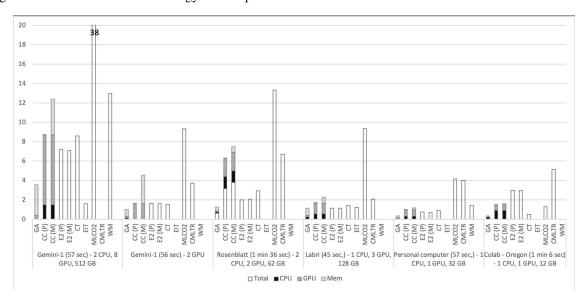
Figure 1: Energy consumption in Wh of the different methods over the 5 different infrastructures for the first experiment. For the tools that do not provide detail for CPU/GPU/Memory consumption, the total energy reported is plotted.
