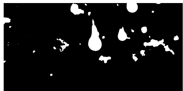
Figure 5: Thresholding following the Top-hat transform application on the image of the P1 propellant at the initial pressure of 5 bar .
