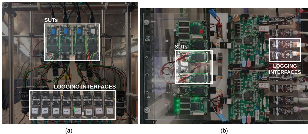
Fig. 3: Experimental setups prepared for irradiation campaigns. **(a) Chiplr: six test boards, in two layers, and logging interfaces (highlighted).** **(b) CHARM: two test boards, in parallel, and logging interfaces (highlighted).**
