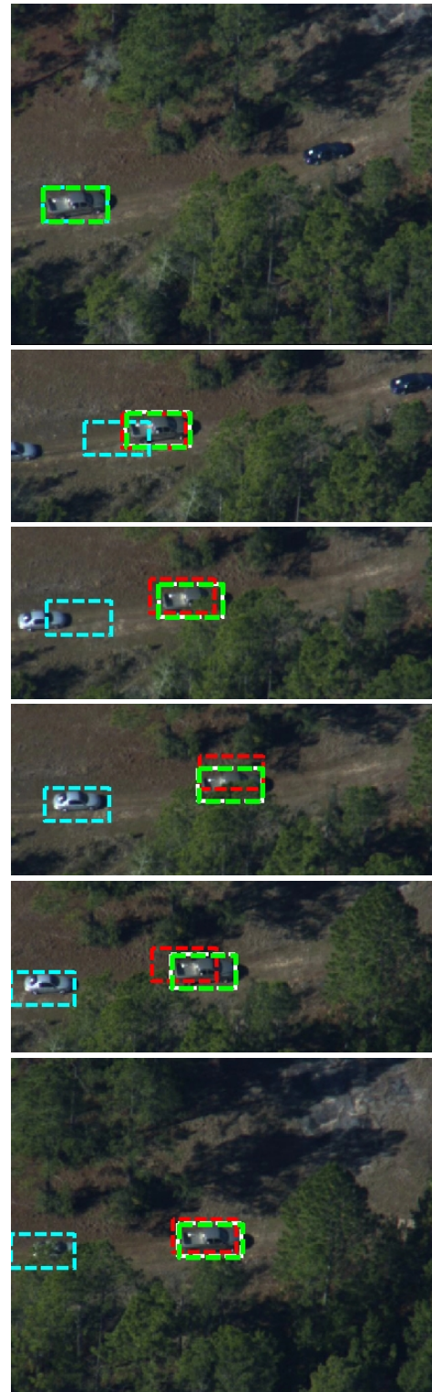
Figure 2. Tracking on sequence “Car”: frames 1, 30, 60, 90, 120 and 150 (relative to the reference frame). kNN-KL-G (proposed method): green; kNN-KL: cyan; Mean-shift: red; SAD: white. The car is partially occluded by trees from frame 36 to frame 116. \Omega : 95×47-rectangle.
