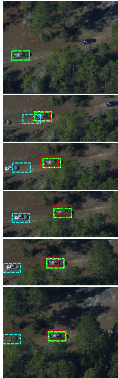
Figure 2. Tracking on sequence “Car”: frames 1, 30, 60, 90, 120 and 150 (relative to the reference frame). kNN-KL-G (proposed method): green; kNN-KL: cyan; Mean-shift: red; SAD: white. The car is partially occluded by trees from frame 36 to frame 116. \Omega : 95 \times 47 -rectangle.
