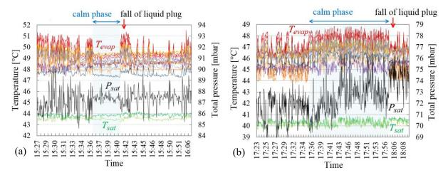
**Figure 8.** Examples of temperature and pressure signatures of an intermittent "liquid motions" regime (a) water, charge 6,  $d_{in} = 10.7$  mm,  $\dot{Q}_{pc}/\dot{Q}_{tot} = 64 / 95$  W, (b) water, charge 6,  $d_{in} = 7.6$  mm,  $\dot{Q}_{pc}/\dot{Q}_{tot} = 51 / 80$  W.
