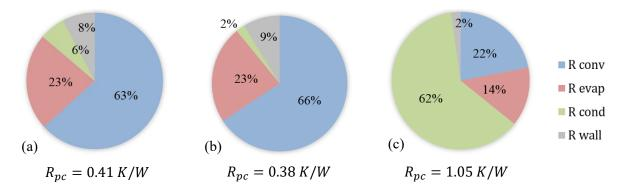
**Figure 11.** Thermal performance of the vapor chamber filled with water. Comparison of relative contributions for various diameters at the highest tested heat load (a)  $d_{in} = 10.7$  mm,  $\dot{Q}_{pc} = 64$  W, (b)  $d_{in} = 7.6$  mm,  $\dot{Q}_{pc} = 70$  W, (c)  $d_{in} = 5.3$  mm,  $\dot{Q}_{pc} = 36$  W.
