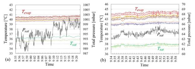
**Figure 5.** Examples of temperature and pressure signatures of a stable oscillatory regime (a) pentane, charge 5,  $d_{in} = 5.3$  mm,  $\dot{Q}_{pc}/\dot{Q}_{tot} = 55 / 75$  W, (b) water, charge 10,  $d_{in} = 10.7$  mm,  $\dot{Q}_{pc}/\dot{Q}_{tot} = 52 / 80$  W.
