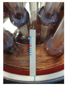
**Figure 2.** Scaled ruler for fluid charge measurement through the condenser base plate.
