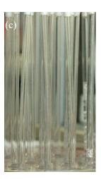
**Figure 4.** Illustrations of condensation regimes (a) pentane filmwise condensation, (b) water liquid plug and dropwise condensation inside a 7.6 mm diameter fin, (c) 5.3 mm diameter fins filled with stable water plugs.
