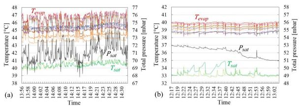
**Figure 7.** Examples of temperature and pressure signatures of an intermittent "boiling" regime (a) water, charge 5,  $d_{in} = 10.7$  mm,  $\dot{Q}_{pc}/\dot{Q}_{tot} = 51 / 80$  W, (b) water, charge 6,  $d_{in} = 10.7$  mm,  $\dot{Q}_{pc}/\dot{Q}_{tot} = 20 / 40$  W.
