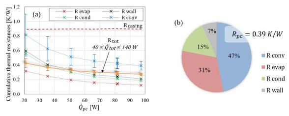
**Figure 10.** Thermal performance of the vapor chamber filled with HFE-7100 (constant fluid fill charge optimized for the highest tested heat load) for  $d_{in} = 5.3$  mm (a) evolution of the cumulative thermal resistances with the heat load  $\dot{Q}_{pc}$  and comparison of  $R_{tot}$  and  $R_{casing}$ , (b) comparison of relative contributions for the highest tested heat load  $(\dot{Q}_{pc}/\dot{Q}_{tot} = 97/140 \text{ W})$ .
