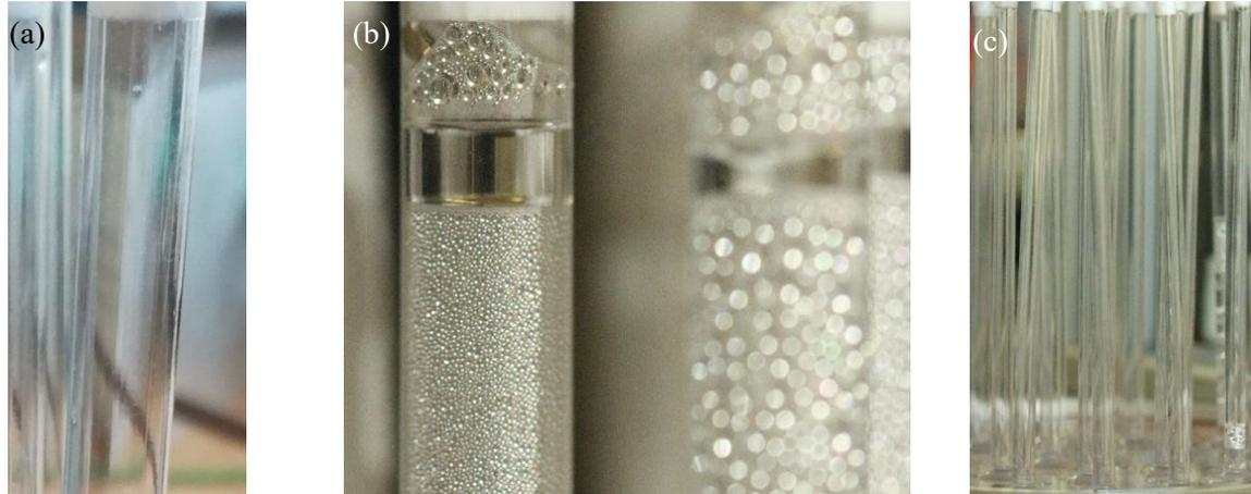
**Figure 4.** Illustrations of condensation regimes (a) pentane filmwise condensation, (b) water liquid plug and dropwise condensation inside a 7.6 mm diameter fin, (c) 5.3 mm diameter fins filled with stable water plugs.
