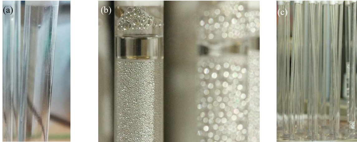
Figure 4. Illustrations of condensation regimes (a) pentane filmwise condensation, (b) water liquid plug and dropwise condensation inside a 7.6 mm diameter fin, (c) 5.3 mm diameter fins filled with stable water plugs.
