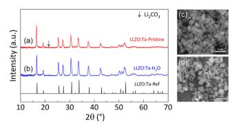
Figure 1. XRD patterns of a) pristine LLZO:Ta and b) water-treated LLZO: Ta-H<sub>2</sub>O compared to the reference pattern of LLZO:Ta. SEM images of c) pristine LLZO:Ta and d) water-treated LLZO:Ta-H<sub>2</sub>O.
