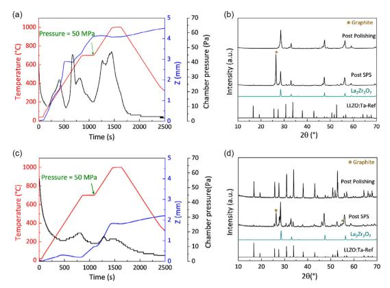
**Figure 4.** SPS protocol and collected displacement of punches and pressure of the chamber during the processing of a) the pristine LLZO: Ta powder and b) the argon-pretreated powder. Experimental XRD pattern of the densified pellet after the SPS process and after polishing compared to the calculated ones for LLZO: Ta reference and  $La_2Zr_2O_7$  c) pristine LLZO: Ta powder and d) the argon pretreated powder.
