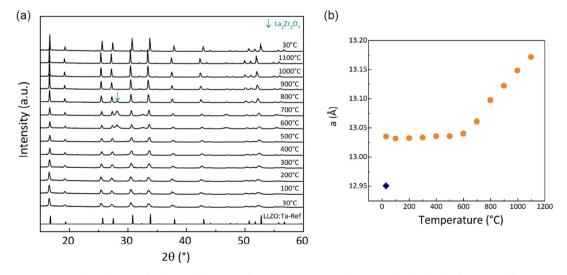
**Figure 2.** a) XRD patterns collected operando during the heating of pristine LLZO:Ta and compared with calculated patterns of LLZO:Ta and  $La_2Zr_2O_7$  b) Evolution of refined lattice parameter of garnet structure as a function of temperature.
