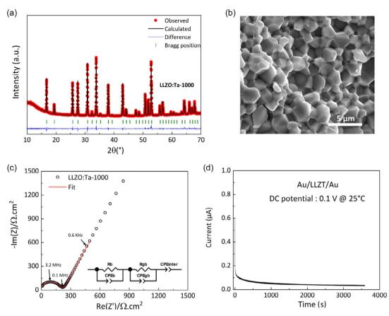
**Figure 5.** a) Rietveld refinement results of the XRD pattern of the pellet sintered at 1000 °C b) Cross-section SEM image of the LLZO:Ta sintered ceramic. c) Nyquist plot for the electrochemical impedance of LLZO:Ta densified by SPS at 1000 °C placed between two Au blocking electrodes and the corresponding fit with the equivalent circuit. d) The current-time curve of the Au/LLZO:Ta/Au cell under DC polarization at different potentials.
