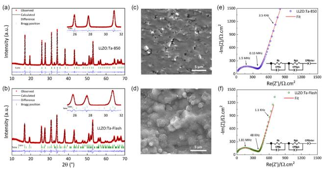
Figure 6. a,b) Rietveld refinement results of the XRD patterns; c,d) cross-section SEM images, and e) Nyquist plot of the impedance with the corresponding equivalent circuit, f) of respectively the LLZO:Ta pellet sintered at 850 °C and the pellet sintered using the Flash-SPS process.
