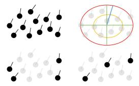
Fig. 3 The display types of the swarm (from [32]): in the top left, the *full information* display, *i.e.* each agent's direction; in the top right, the swarm's centroid (at the intersection of the green cross), along with a bounding ellipse (in red) and another ellipse (in yellow) representing the robot positions median; and in the bottom left and right, only some leaders' direction.
