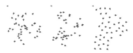
Fig. 2 Robot swarm simulation used in the evaluation of *Neglect Benevolence* (from [33]). At the initial state (a), each robot follows its own randomly generated heading. The middle section (b) shows the robots after they have self-organised to follow the same direction. Section (c) shows the robots after the reception of the operator's command to coordinate their movement.
