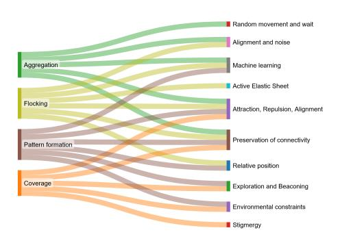
Fig. 6 Sankey diagram of four emergent robot swarms' elementary behaviours (left) that can be obtained through the use of self-organisation methods (right). From [15].
