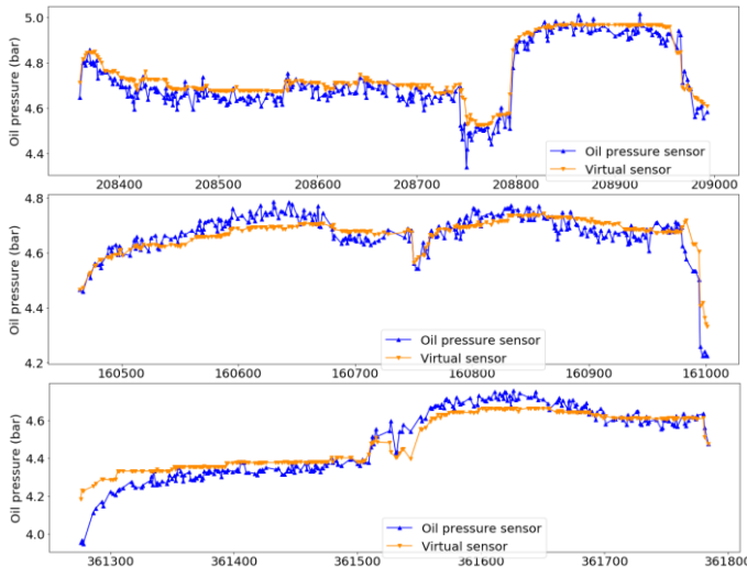
Figure 9: Oil pressure sensor (blue line) and virtual sensor (orange line) for three normal flights
