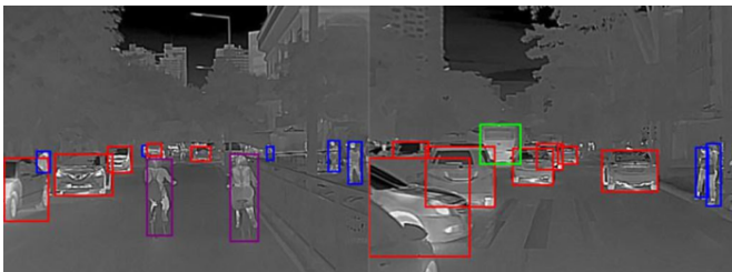
Fig. 7. Object detection in thermal images. Pedestrians, vehicles, etc are localized in 2D bounding boxes with different colors. (from [62]).
