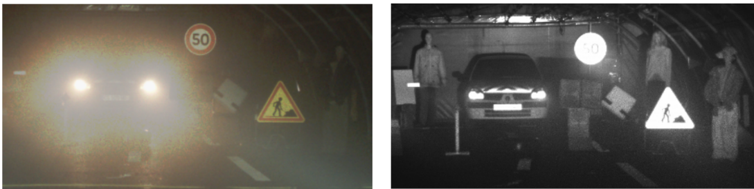
Fig. 9. Imaging results of a conventional RGB camera (left) and a range-gated camera (right) in an artificial fog (from [137]). Due to the backscattering effect caused by the fog, many objects are obscured in the RGB camera image, while the range-gated camera image is almost immune to the fog. Meanwhile, the headlamp of the target car causes a strong blooming effect in the RGB camera image but has no impact on the range-gated camera image.
