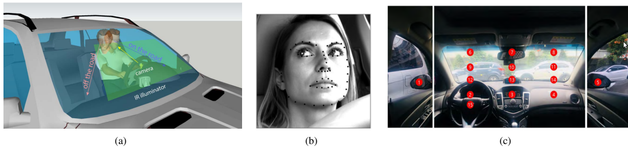
Fig. 5. (a) An example of a DMS consisting of a camera and an IR illuminator facing the driver to detect whether the driver’s eyes are on the road or not (from [76]). (b) Face landmark detection results (from [77]). (c) 15 zones for gaze classification (from [78]).
