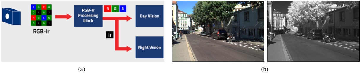
Fig. 3. (a) A RGB-IR imaging system: the CFA is replaced by an RGB-IR filter array to capture RGB and infrared intensities (from [26]) (b) RGB (left) and NIR (right) images for the same scene. Vegetation in the NIR spectrum is “brighter” than in RGB image (from [27]).
