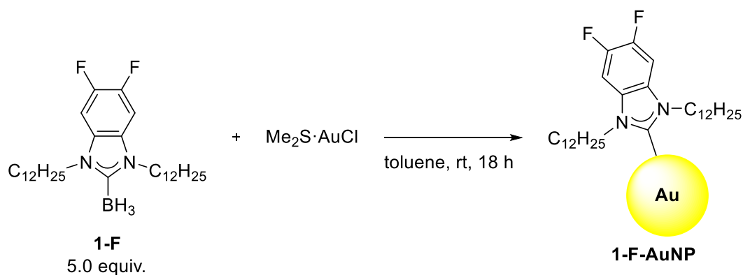
Scheme 4. Synthesis of nanoparticles 1-F-AuNPs from NHC-borane 1-F .
