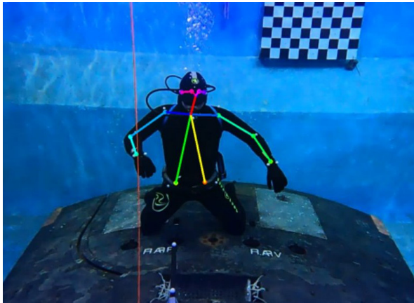
Fig. 2: Skeleton detection on underwater image using OpenPose [13]
