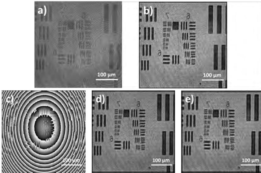
**Figure 2.** a) Example of a Digital hologram registered with a DHM set-up. In focus image restitution of an USAF test target at a distance of 81  $\mu\text{m}$  b) in amplitude c) in phase, with spherical aberrations. Defocus images reconstructed at distances of d) 121  $\mu\text{m}$  and e) 161  $\mu\text{m}$ .
