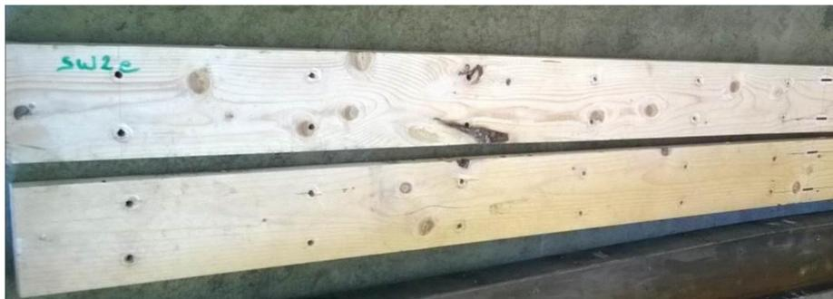
**Figure 4: example of timber elements used in hybrid beam tests in the study**
