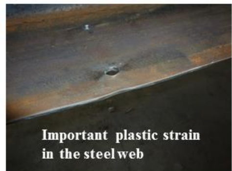
Figure 17: behavior of beam SW3 (configuration II – arrangement v1)
