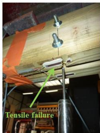
Figure 15: experimental setup with load-displacement and load-strain curves of beam SW4B
