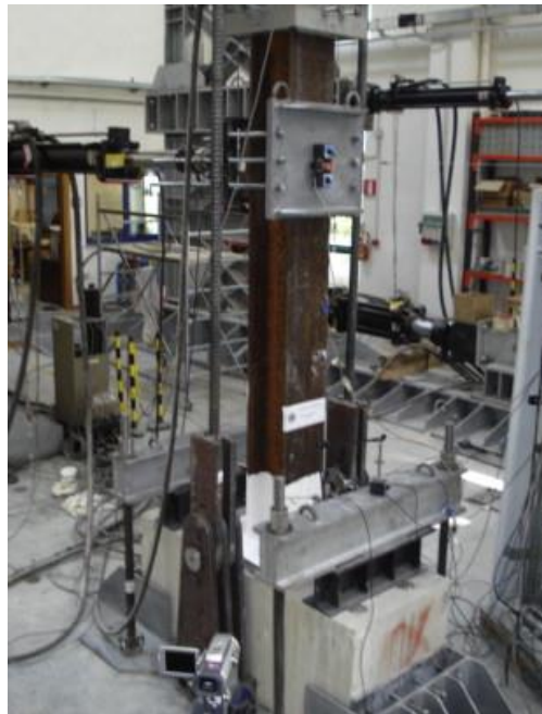
Figure 2. Column base connection test setup [9]
