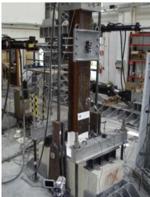
Figure 2. Column base connection test setup [9]
