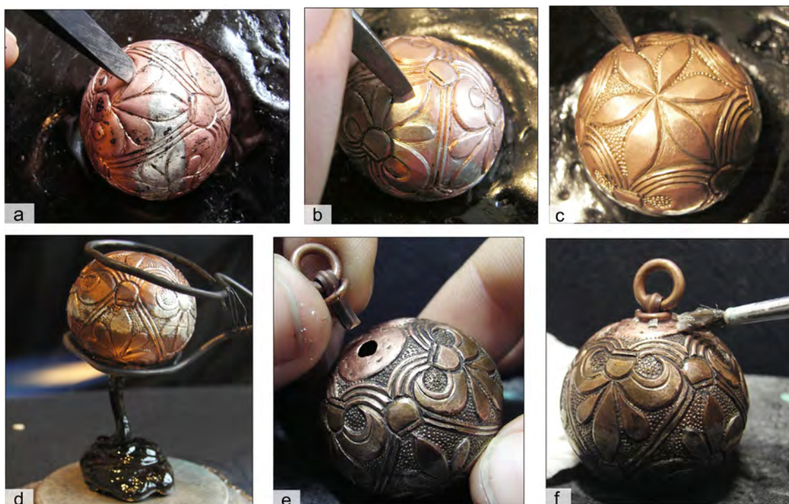
Fig. 13 Manufacture of a replica of gombik 217/8 by the professional goldsmith Ludmila Barčáková. a Chasing of the palmette motive with a narrow chasing tool, note the smeared Ag-Cu hard solder around the joining area. b Working on the edge and plane surface with a planishing
