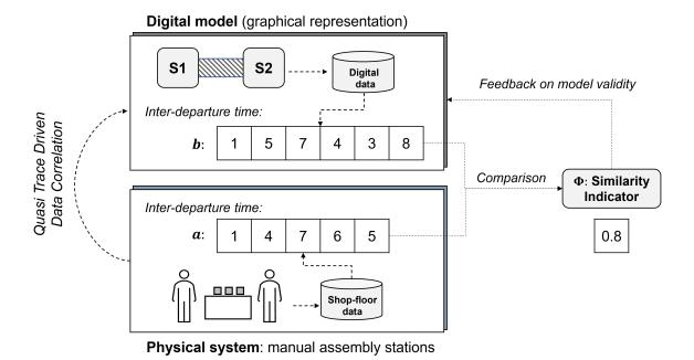
Fig. 1: Example - Comparison of data sequences generated by a real system composed by two manual assembly stations and its corresponding digital model. The inter-departure times are collected from the physical system (a) and measured also in the digital space (b). A similarity indicator is used to assess the validity of the digital model.
