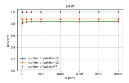
Fig. 12: Experiments – Logic validation at performance-level: 95% confidence intervals of the DTW-based indicator (KPI: *system time*).
