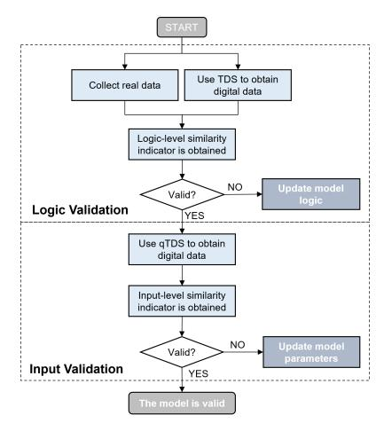
Fig. 3: Proposed online validation procedure (TDS: Trace Driven Simulation; qTDS: quasi Trace Driven Simulation).
