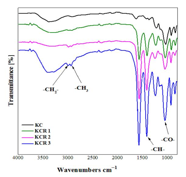
Figure 2. FTIR spectra of kappa carrageenan and its derivative KCRs.
