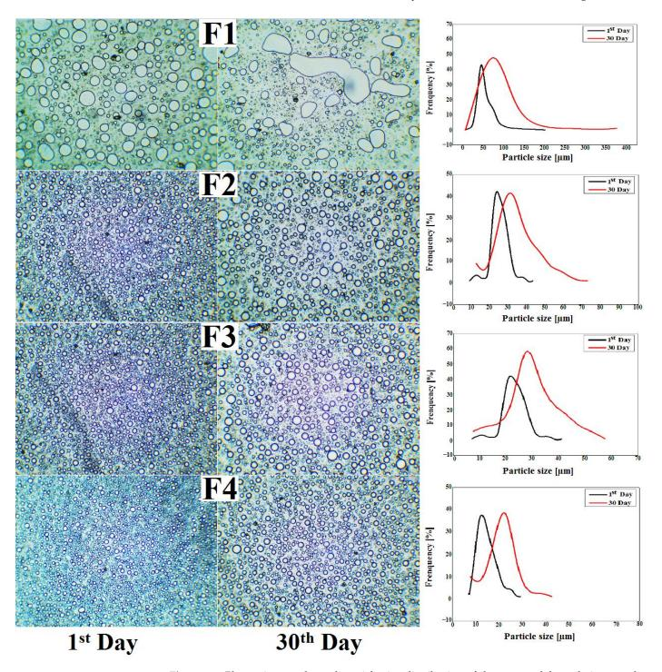
**Figure 11.** Photomicrographs and particle size distribution of the prepared formulations on the 1st day and the 30th day. Micrographs with a magnification of 10×: Emulsions F1, F2, F3, and F4 stabilized by KC, KCR1, KCR2, and KCR3 derivatives, respectively, at 1%.
