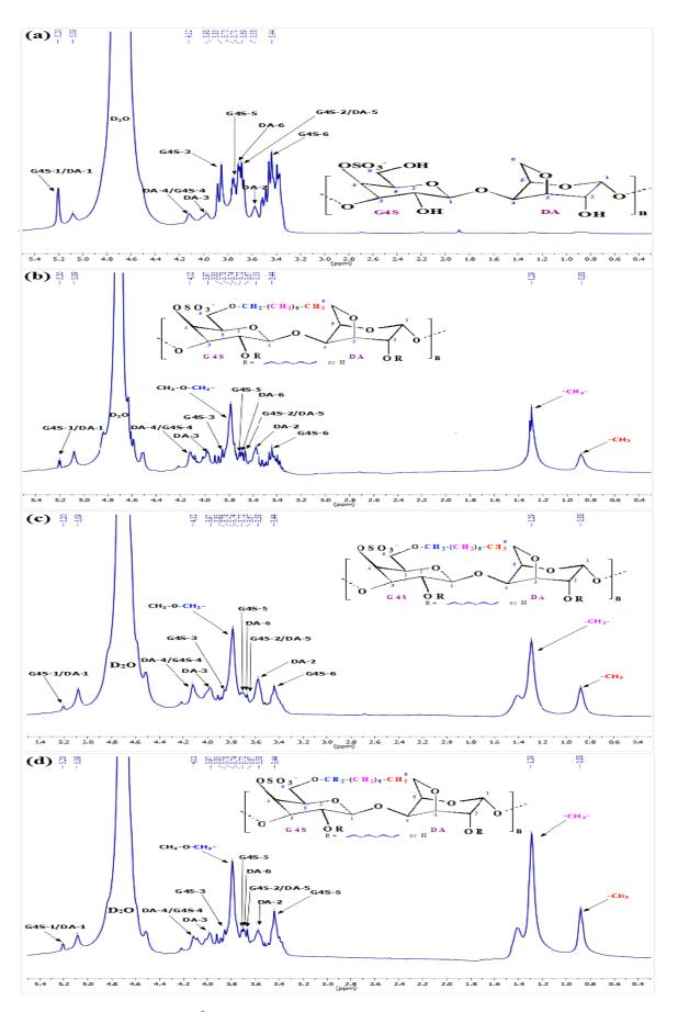
Figure 3. <sup>1</sup>HNMR spectra of kappa carrageenan (a), KCR1 (b), KCR2 (c), and (c) KCR3 (d).
