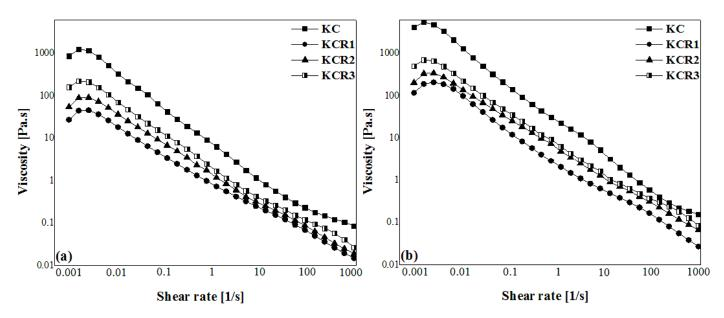
**Figure 7.** Flow curves of native kappa carrageenan, and its derivative KCRs at concentrations of 0.75% (**a**) and 1% (**b**).
