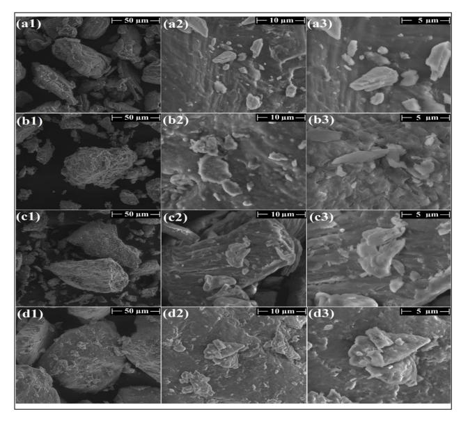
**Figure 5.** SEM micrographs of KC (**a1–a3**), KCR1 (**b1–b3**), KCR2 (**c1–c3**), and KCR3 (**d1–d3**) at different magnifications. From left to right: 50  $\mu$ m, 10  $\mu$ m, 5  $\mu$ m, and 1000×, 6000×, 16,000×.
