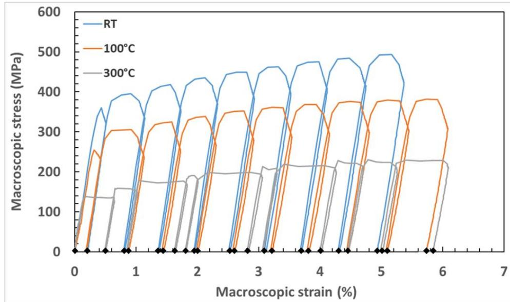
Figure 2: Experimental macroscopic stress-strain curves at RT, 100 and 300°C. The black points indicate the macroscopic strain during neutron measurements after unloading, i.e. at zero applied load.
