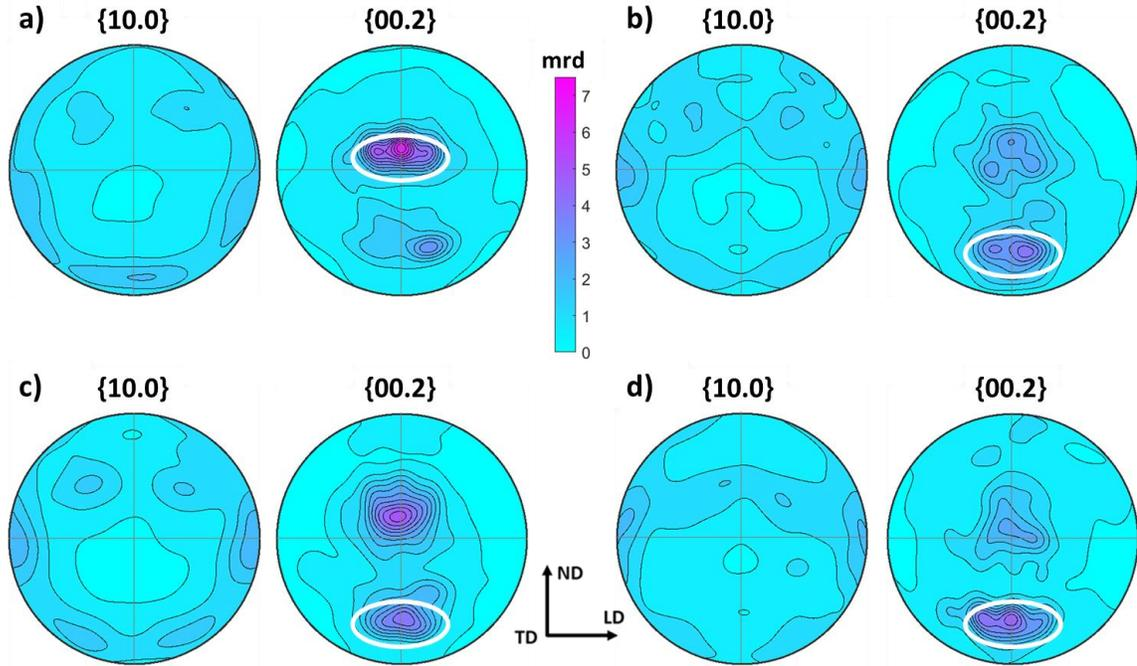
Figure 1: crystallographic textures of the studied specimens. As-received samples (a), after the tensile loading up to 6 %: at room temperature (b), at 100°C (c) and at 300°C (d).  $\{10.0\}$  and  $\{00.2\}$  PFs are represented in the LD-ND plane. ND: Normal Direction, TD: Transverse Direction, LD: Longitudinal Direction.
