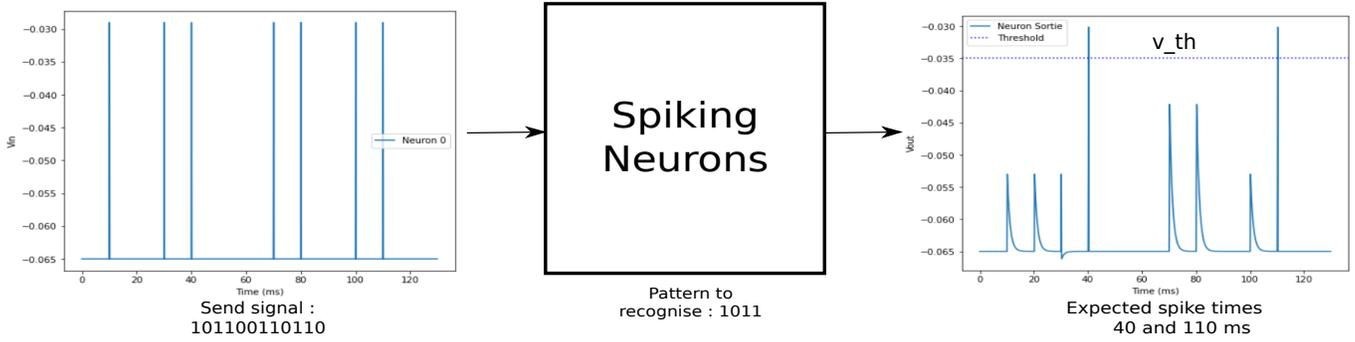
Fig. 2. Ideal input and output of the SNN.
