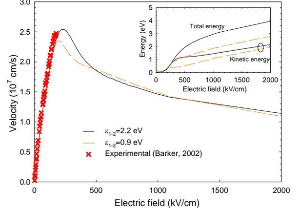
Fig. 6. Average velocity of electrons vs. electric field,  $E$ , for GaN doped at  $N_D=5 \times 10^{18}$  cm $^{-3}$  at room temperature for  $\epsilon_{1-2}=2.2$  and 0.9 eV compared with the experimental measurements of [51]. The inset shows the average total and kinetic energies vs.  $E$ .
