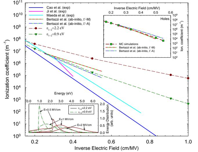
Fig. 5. Ionization coefficients vs. inverse electric field obtained with MC simulations using  $\epsilon_{th}=3.5$  eV,  $k=4$ , and  $S=10^{13}$  s $^{-1}$ , for intervalley energy separations of  $\epsilon_{1-2}=2.2$  and 0.9 eV. The insets show the impact ionization coefficient for holes and the distribution function of the total energy for electric fields of 0.5, 1.0 and 2.0 MV/cm.
