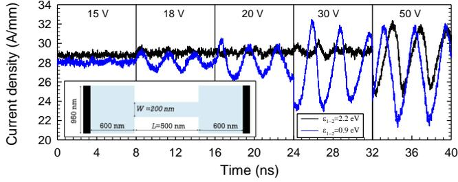
Fig. 7. Time-sequences of current density for a 200 nm wide 0.5  $\mu\text{m}$  long GaN channel (geometry shown in the inset), doped at  $N_D=5\times 10^{18}\text{ cm}^{-3}$ , for applied biases of  $V=15, 18, 20, 30$  and  $50\text{ V}$ , considering  $\epsilon_{1-2}=2.2$  and  $0.9\text{ eV}$ . The inset shows the geometry of the top-view simulations of the n-doped GaN channel.
