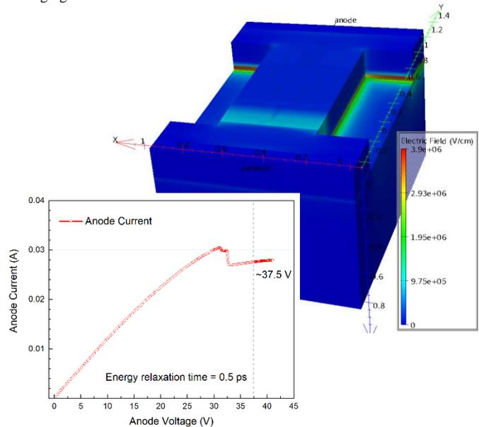
Fig. 4.  $I$ - $V$  curve and 3D map of the electric field of a GaN rectangular channel 500 nm wide and 1.0  $\mu\text{m}$  long, doped at  $N_D=2 \times 10^{18}$   $\text{cm}^{-3}$ , for an applied bias of  $V=37$  V (above the onset of Gunn oscillations). Results obtained with the commercial TCAD Silvaco ATLAS simulator using the Energy Balance model.
