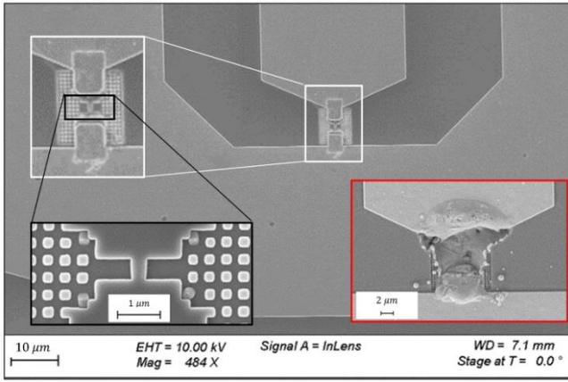
Fig. 1. SEM picture of a fabricated diode formed of a tapered channel with  $W_i=300$  nm,  $W_o=350$  nm and  $L=0.5$   $\mu$ m. The bottom right picture shows a diode after its catastrophic failure, where anode and cathode are short-circuited by the melted metallic pads.
