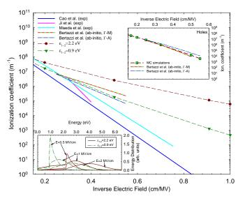
Fig. 5. Ionization coefficients vs. inverse electric field obtained with MC simulations using  $\epsilon_{th}$ =3.5 eV, k=4, and S=10<sup>13</sup> s<sup>-1</sup>, for intervalley energy separations of  $\epsilon_{1-2}$ =2.2 and 0.9 eV. The insets show the impact ionization coefficient for holes and the distribution function of the total energy for electric fields of 0.5, 1.0 and 2.0 MV/cm.
