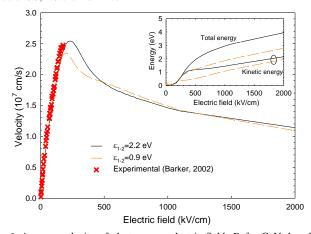
Fig. 6. Average velocity of electrons vs. electric field, E, for GaN doped at  $N_D$ =5×10<sup>18</sup> cm<sup>-3</sup> at room temperature for  $\varepsilon_{1-2}$ =2.2 and 0.9 eV compared with the experimental measurements of [51]. The inset shows the average total and kinetic energies vs. E.
