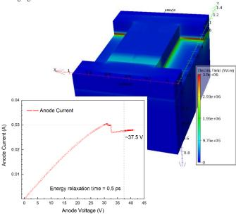
Fig. 4. *I-V* curve and 3D map of the electric field of a GaN rectangular channel 500 nm wide and 1.0  $\mu$ m long, doped at  $N_D$ =2×10<sup>18</sup> cm<sup>-3</sup>, for an applied bias of V=37 V (above the onset of Gunn oscillations). Results obtained with the commercial TCAD Silvaco ATLAS simulator using the Energy Balance model.
