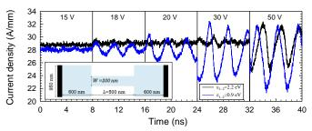
Fig. 7. Time-sequences of current density for a 200 nm wide 0.5  $\mu$ m long GaN channel (geometry shown in the inset), doped at  $N_D$ =5×10<sup>18</sup> cm<sup>-3</sup>, for applied biases of V=15, 18, 20, 30 and 50 V, considering  $\varepsilon_{1-2}$ =2.2 and 0.9 eV. The inset shows the geometry of the top-view simulations of the n-doped GaN channel.
