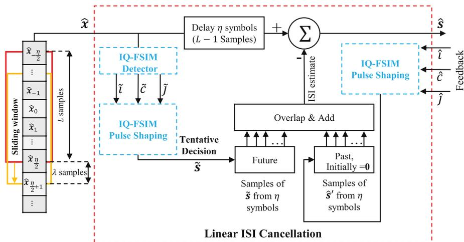
**Fig. 3** ISI estimation and cancellation (ISI-EC) for IQ-FSIM. The causal ISI is compensated in ISI-EC by using the feedback final decisions  $\{\hat{i}, \hat{j}, \hat{c}\}$  for past symbols, while the causal ISI is estimated by tentative detection of  $\{\tilde{i}, \tilde{j}, \tilde{c}\}$  for future symbols
