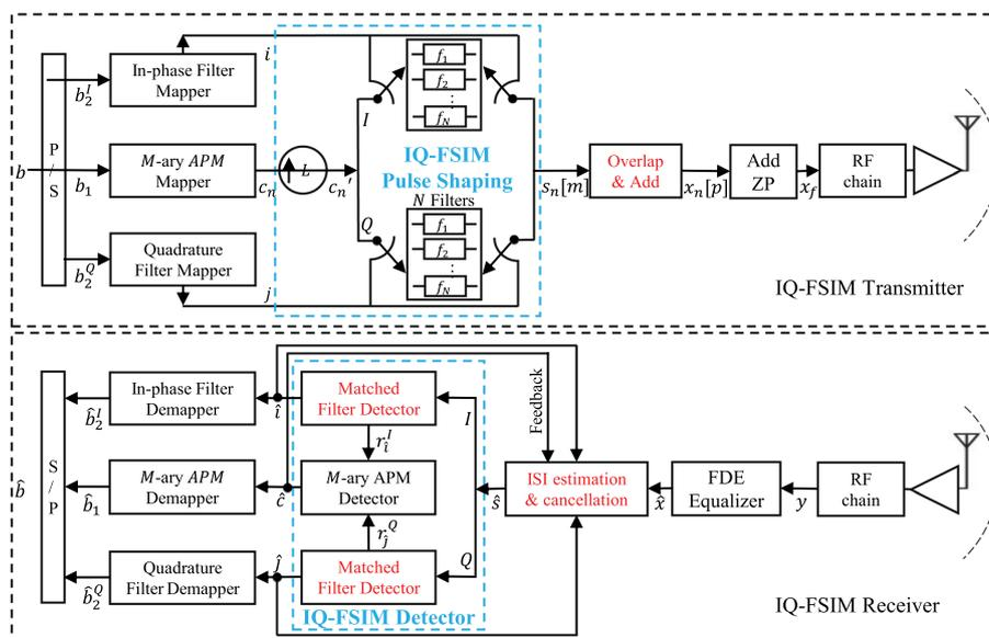
**Fig. 1** Block diagram of the proposed IQ-FSIM transceiver
