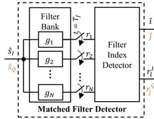
**Fig. 2** Matched filter-based detector for IQ-FSIM. This block estimates the index  $\hat{i}$  ( $\hat{j}$ ) of the filter shape being used at I (Q) component using the input  $\hat{s}^I$  ( $\hat{s}^Q$ )
