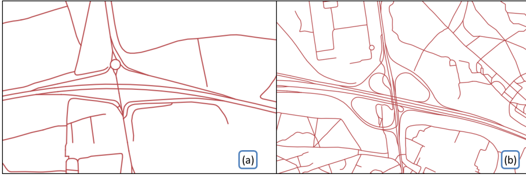
Figure 7: Two examples of a highway interchange structure, a simple one on the left, and a more complex one on the right, illustrating the difficulty to clearly define what this structure is.
