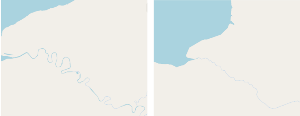
Figure 2: Generalisation of the Seine River in OpenStreetMap multi-scale maps (with all other themes removed for more clarity) between zoom levels 7 and 6. The meanders of the Seine are no longer recognizable after application of a smoothing algorithm.
