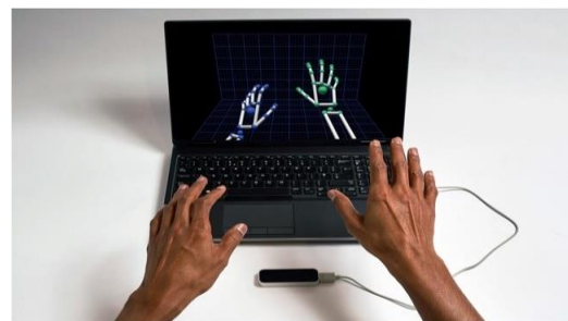
Figure 1. The Leap Motion hand capture device and graphic rendering of points of interest (from ultraleap.com)
