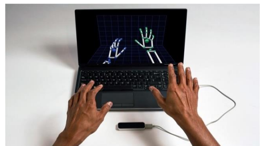
Figure 1. The Leap Motion hand capture device and graphic rendering of points of interest (from ultraleap.com)
