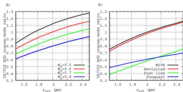
**Figure A3.** Theoretical IR/Vis AOD coarse-mode ratio as a function of the effective radius (a) for the MITR model and the standard deviation of the width of the size distribution  $\sigma_g$ , (b) for  $\sigma_g = 0.6$  and several refractive indices.
