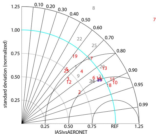
**Figure 2.** Taylor diagram (normalized) for IASI and AERONET 500 nm coarse-mode AOD over oceanic regions. Sites are identified by their number in Table 2. Grey numbers are for “Level 1.5” sites. The overall statistics appear in blue (“av” for average). Correlation shown on the external circle; amplitude: radial distance.
