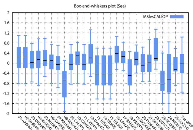
**Figure 7.** Box-and-whiskers plot (ends of the whiskers exclude the outliers) for the difference between IASI and CALIOP altitude over oceanic regions. y axis is in kilometres. Sites are identified by their number and code as defined in Table 4, followed by the number of items. Last box: overall result. NB: a systematic bias of  $-0.4$  km (IASI–CALIOP) has been removed from the mean (all sites and total).
