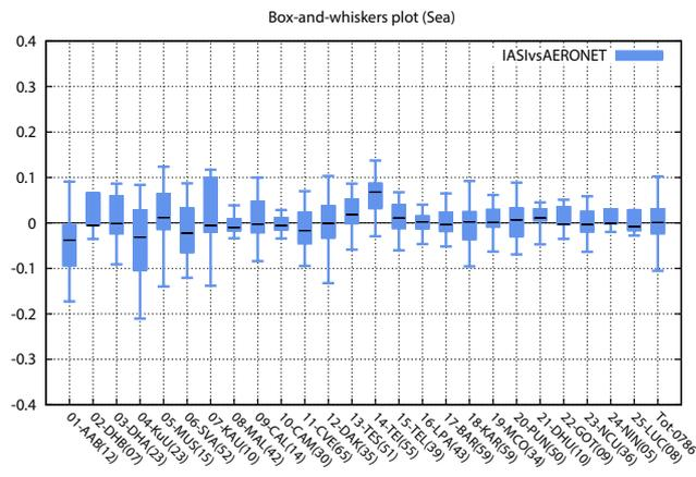
**Figure 3.** Box-and-whiskers plot (ends of the whiskers exclude the outliers) for the difference between IASI and AERONET 500 nm coarse-mode AOD (scaled by the site ratio as explained in Sect. 3) over oceanic regions. Sites are identified by their number and code in Table 2, followed by the number of items. Last box marked “Tot”: overall result.
