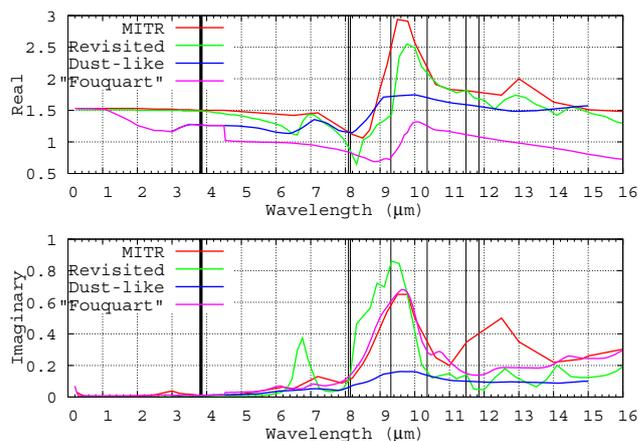
**Figure A2.** Real (top) and imaginary (bottom) refractive index for the MITR model (Hess et al., 1998; Volz, 1973) in red; the “revisited” (Balkanski et al., 2007) model in green; the “dust-like” model from Volz (1972, 1973) in blue, and “Fouquart” et al. (1987) in pink. Black vertical bars indicate the location of the IASI channels used in the aerosol retrieval.
