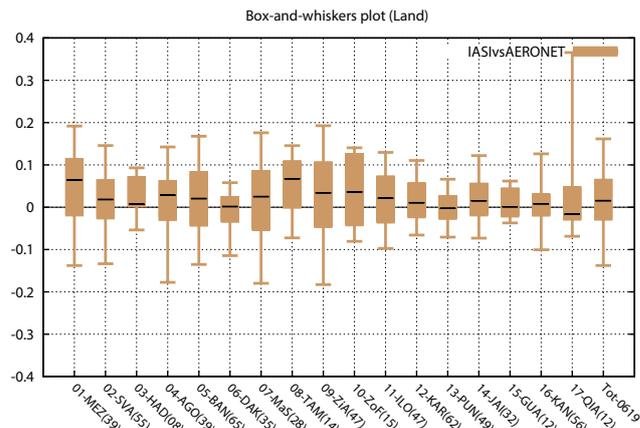
**Figure 5.** Box-and-whiskers plot (ends of the whiskers exclude the outliers) for the difference between IASI and AERONET 500 nm coarse-mode AOD (scaled by the site ratio as explained in Sect. 3) over land. Sites are identified by their number and code in Table 3, followed by the number of items. Last box marked “Tot”: overall result.
