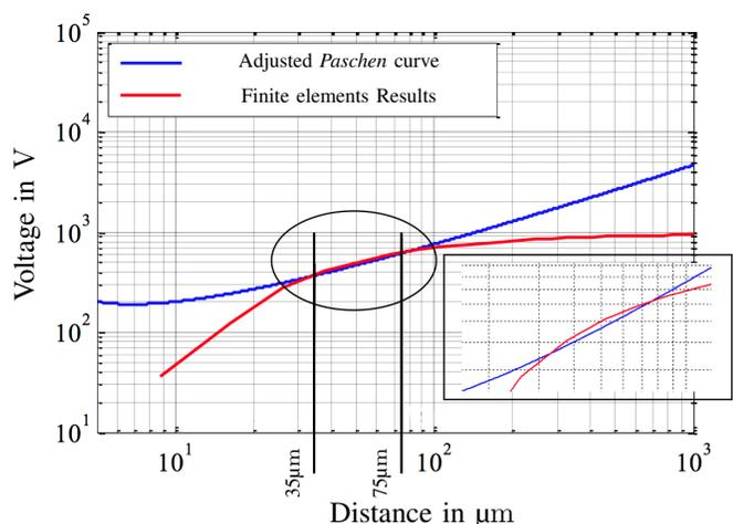
Fig. 6: Localisation of partial discharges critical area
