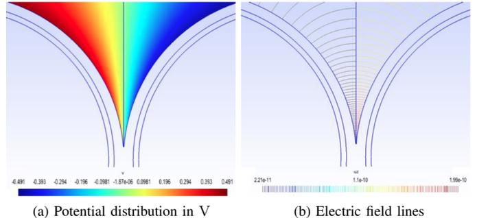
Fig. 4: Results of the finite elements simulation
