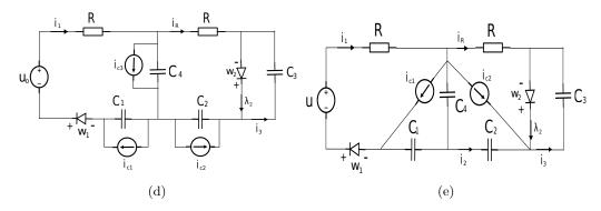
Figure 22: RLCD circuit with two ideal diodes and both voltage and current sources.
