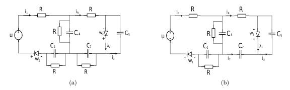
Figure 21: RLCD circuit with two ideal diodes.
