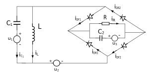
Figure 28: Diode Bridge
