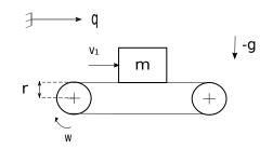
Figure 30: Simple mechanical system with Coulomb's friction.
