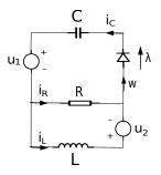
Figure 15: RLCD circuit with one ideal diode.
