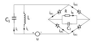
Figure 27: Diode Bridge
