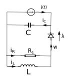
Figure 17: RLCD circuit with current source
