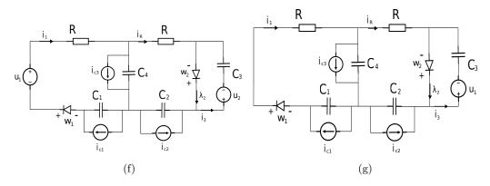
Figure 24: RLCD circuit with two ideal diodes and both voltage and current sources.
