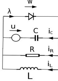
Figure 26: RLCD circuit
