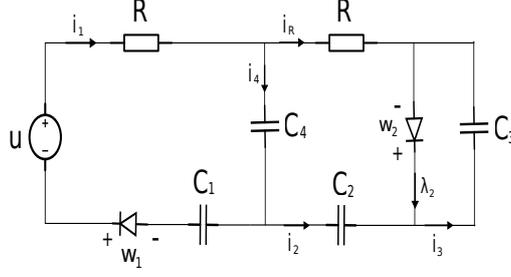
Figure 20: RC circuit with two ideal diodes
