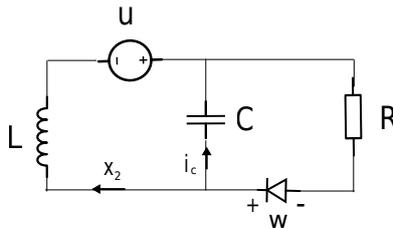
Figure 12: RLCD circuit with one ideal diode.
