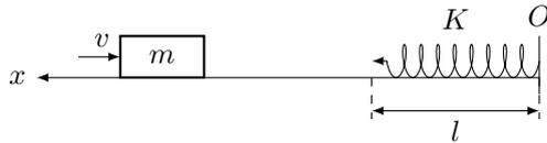
Figure 29: Mechanical system with unilateral spring.
