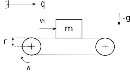
Figure 30: Simple mechanical system with Coulomb's friction.
