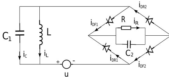
Figure 27: Diode Bridge
