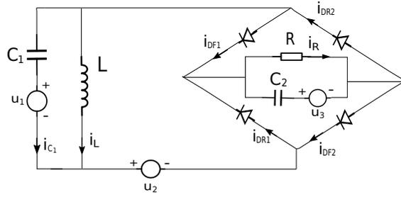
Figure 28: Diode Bridge
