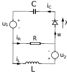
Figure 15: RLCD circuit with one ideal diode.
