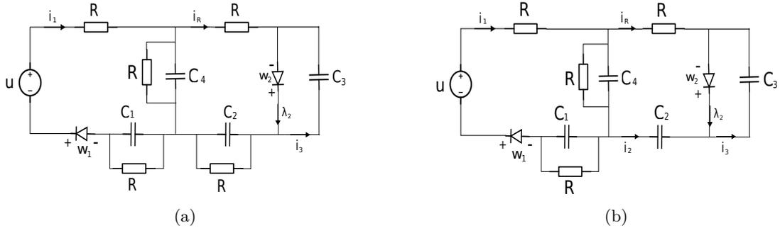
Figure 21: RLCD circuit with two ideal diodes.
