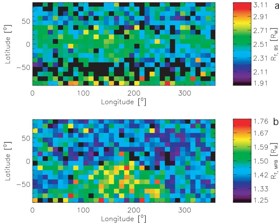
**Fig. 8.** Longitude-latitude maps colour coded by the extrapolated terminator distance  $R_T$  of the (a) BS and (b) MPB as observed by MEX. Only dayside crossings were used. Black bins means that there were less than two crossings in that region.
