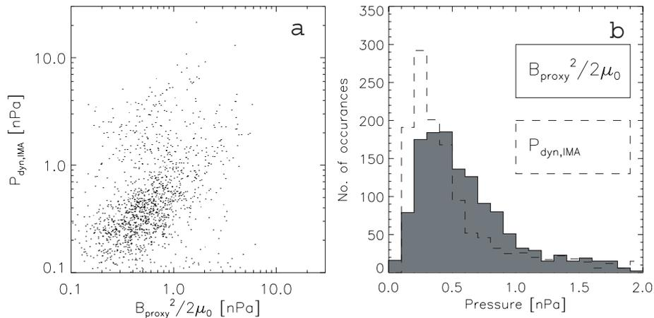
**Fig. 1.** (a) Measured solar wind dynamic pressure from MEX/IMA plotted vs. the MGS proxy for solar wind dynamic pressure and (b) distributions of the MGS proxy and the measured dynamic pressure from MEX/IMA.
