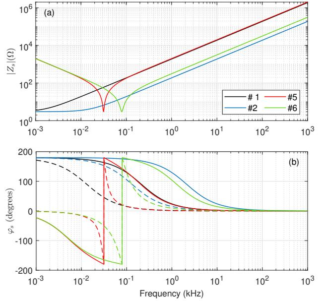
Fig. 3: Comparison of converter station models: (a) modulus of the input impedance for four different models (cf. Table I); (b) phase-shift angle  $\varphi_s$  of the reflection coefficient, assuming an OHL (solid lines) or a CCL (dashed lines).
