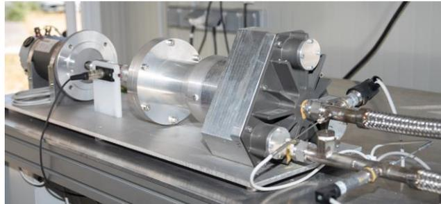
Figure 7- Scroll expander implemented in the prototype.
