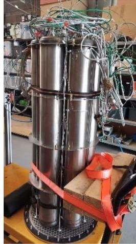
Figure 6- Tube-calendar reactor with the 7 tubes reactors connected together.
