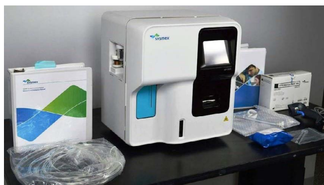
Figure 2 Sysmex XP 100- (Sysmex Corp., Hyogo, Japan) for evaluation of complete blood picture including platelet counts.
