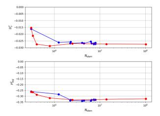
Figure B1. Evolution of the global molecular dissipation,  $D_{\nu}^{V}$  (top), and the global transfer to TKE,  $P_{\text{TKE}}^{V}$  (bottom) as a function of the number of elements,  $N_{\text{elem}}$  during the automatic mesh convergence procedure based on LIKE criterion (red line) and based on  $QC_1$  and  $QC_2$  criteria (blue line).
