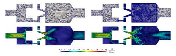
Figure 17. PRECCINSTA configuration. Top: Initial (left) and final (right) meshes of the center plane. Bottom: Center plane colored by the non-dimensional instantaneous velocity norm,  $|\vec{u}|/U_{max}$ , computed on the initial (left) and the final (right) meshes.
