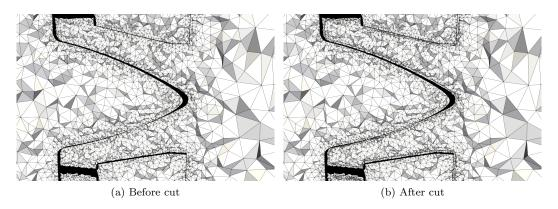
Figure 13. Cutting of the mesh on the level set iso-contour and STL file (black)
