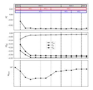
Figure A2. Evolution of the global molecular dissipation,  $D_{\nu}^{\mathcal{V}}$  (top), the global transfer to TKE,  $P_{\text{TKE}}^{\mathcal{V}}$  (middle), and the number of elements,  $N_{\text{elem}}$  (bottom) during the different states of the automatic mesh convergence procedure in the turbulent round jet configuration starting from another initial mesh.
