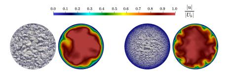
Figure 5. Turbulent pipe flow configuration. Mesh of a cross section and cross section colored by the non-dimensional instantaneous velocity norm,  $|\vec{u}|/U_b$ , for the initial (left) and final (right) meshes.
