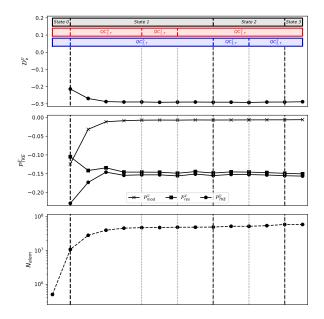
Figure 6. Evolution of the global molecular dissipation,  $D_{\nu}^{\mathcal{V}}$  (top), the global transfer to TKE,  $P_{\text{TKE}}^{\mathcal{V}}$  (middle), and the number of elements,  $N_{\text{elem}}$  (bottom) during the different states of the automatic mesh convergence procedure in the turbulent pipe flow configuration. Note that the resolved,  $P_{\text{res}}^{\mathcal{V}}$ , and the modeled  $P_{\text{mod}}^{\mathcal{V}}$ , parts of the transfer to TKE are also shown.
