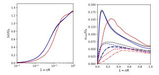
Figure 7. Comparaison of turbulent pipe flow statistics: DNS (black), initial mesh (red) and final mesh (blue). Mean velocity profile (left) and rms velocity profiles (right) for the three directions: axial (solid line), wall-normal (dashed-dotted line) and azimuthal (dashed line).
