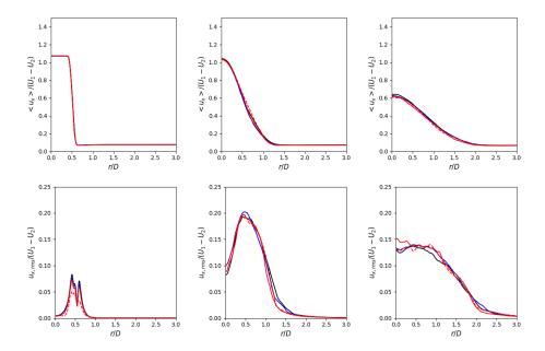
Figure B2. Comparison of turbulent round jet statistics: reference case (black), final mesh for the procedure based on  $QC_1$  and  $QC_2$  criteria (blue), final mesh for the procedure based on LIKE criterion (red, solid line) and the mesh obtained just before (red, dashed line). Mean axial velocity profile (top) and rms axial velocity profile (bottom) at three sections: x/D = 1 (left), 5 (middle) and 10 (right).
