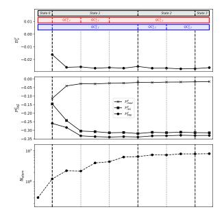
Figure 3. Evolution of the global molecular dissipation,  $D_{\nu}^{\mathcal{V}}$  (top), the global transfer to TKE,  $P_{\text{TKE}}^{\mathcal{V}}$  (middle), and the number of elements,  $N_{\text{elem}}$  (bottom) during the different states of the automatic mesh convergence procedure in the turbulent round jet configuration. Note that the resolved,  $P_{\text{res}}^{\mathcal{V}}$ , and the modeled  $P_{\text{mod}}^{\mathcal{V}}$ , parts of the transfer to TKE are also shown.
