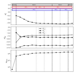
Figure 18. Evolution of the global molecular dissipation,  $D_{\nu}^{\mathcal{V}}$  (top), the global transfer to TKE,  $P_{\text{TKE}}^{\mathcal{V}}$  (middle), and the number of elements,  $N_{\text{elem}}$  (bottom) during the different states of the automatic mesh convergence procedure in the PRECCINSTA burner configuration. Note that the resolved,  $P_{\text{res}}^{\mathcal{V}}$ , and the modeled  $P_{\text{mod}}^{\mathcal{V}}$ , parts of the transfer to TKE are also shown.
