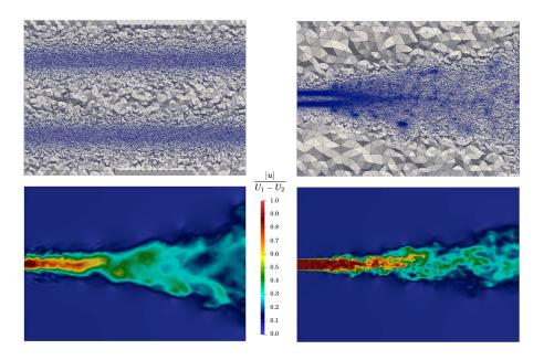
Figure A1. Turbulent round jet configuration starting from another initial mesh. Top: Initial (left) and final (right) meshes of the center plane of the jet flow. Bottom: Center plane colored by the non-dimensional instantaneous velocity norm,  $|\vec{u}|/(U_1 - U_2)$ , computed on the initial (left) and the final (right) meshes.
