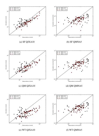
**Fig. 9.** Comparison of the simulated (using SAFRAN/F as atmospheric forcing) and observed QJXA10 and QMNA5. Each dot corresponds to a gauging station. The calculations were made with stations with at least 15 full yr of observed data. Red dots represent the stations that the model simulates reasonably well (NSE > 0.5), black dots correspond to the rest.
