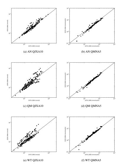
Fig. 12. Comparison of the past and future simulated QJXA10 and QMNA5 for the individual gauging stations.
