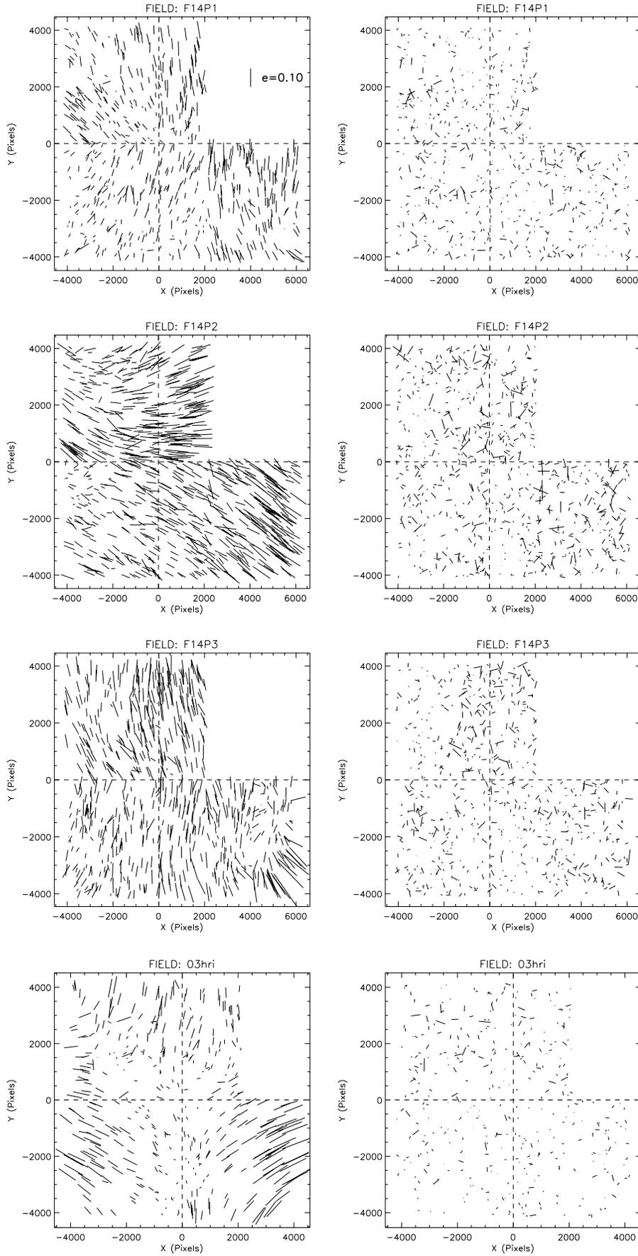
**Fig. 12.** Uncorrected (left) and corrected (right) star ellipticities for FIELD F14P1. The dashed cross shows the location of the optical center. Frames are graduated in pixels. The reference stick at the top-left of the frame shows the amplitude of a 10% distortion. This length of reference applies also for Figs. 13 to 19.
