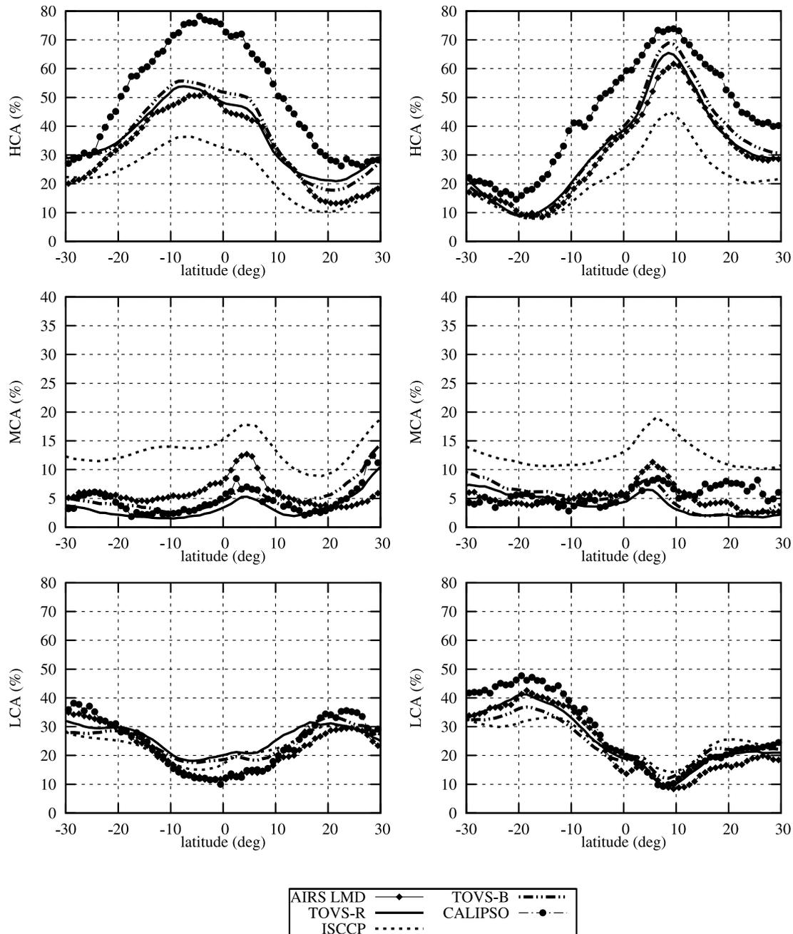
**Figure 10.** Zonal averages of high-cloud amount, midlevel-cloud amount, and low-cloud amount for (left) January and (right) July. Compared are results obtained from the AIRS LMD cloud retrieval (2007), CALIPSO L2 data (2007), TOVS Path-B and reanalyzed TOVS climatological values (1987–1995), and ISCCP climatological values (1987–1995).
