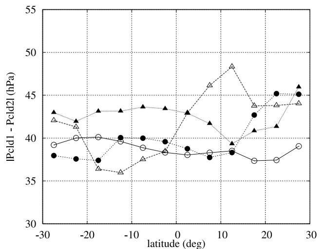
**Figure 8.** Zonal averages of absolute difference between  $p_{\text{cld}}$  of minimum  $\chi_w^2$  and  $p_{\text{cld}}$  of 2. Smallest  $\chi_w^2(p_k)$ , obtained from the LMD AIRS cloud retrieval, separately over ocean (circles) and over land (triangles) and for January 2007 (solid symbols) and for July 2007 (open symbols). This difference gives an estimate of the uncertainty of the retrieved  $p_{\text{cld}}$ .
