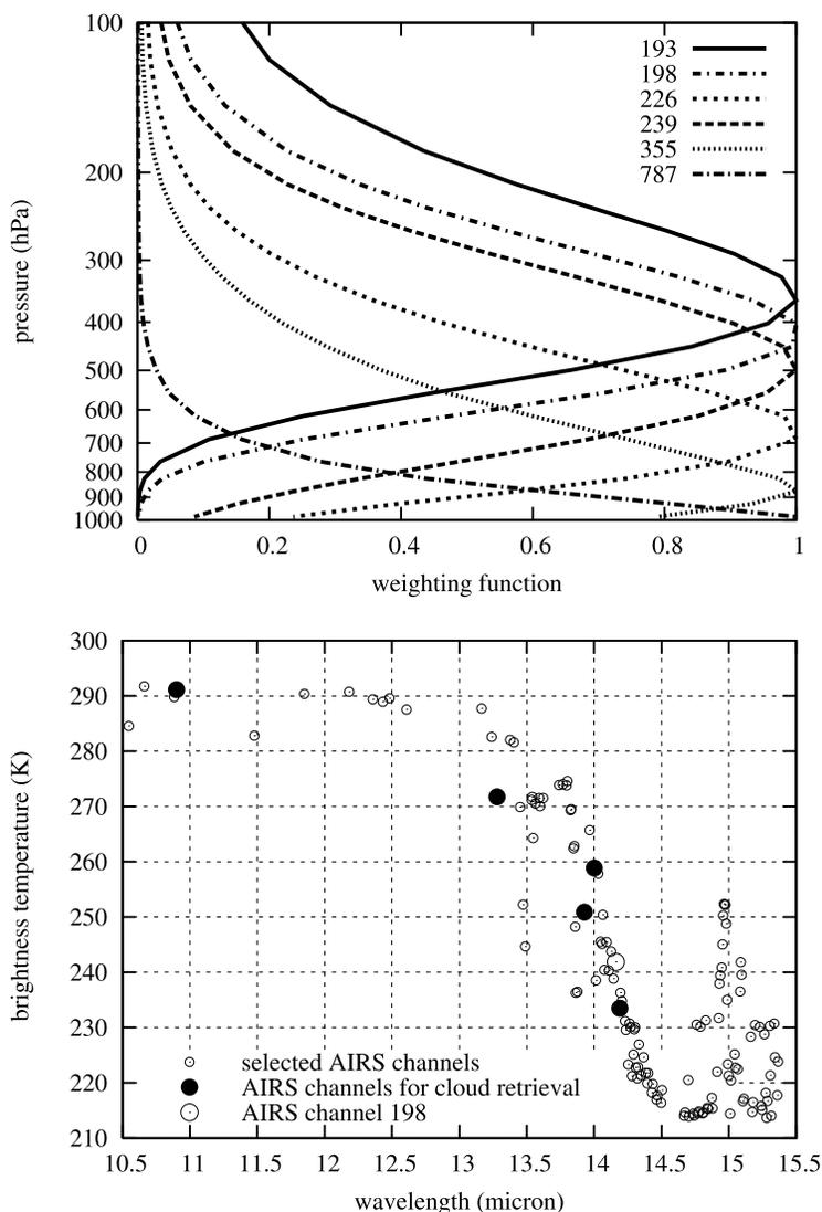
**Figure 1.** (top) Weighting functions of six AIRS channels, around the CO<sub>2</sub> absorption band at 15  $\mu\text{m}$ , used in the cloud property retrieval. (bottom) Simulated clear sky brightness temperature spectrum; the six channels are indicated as big circles.
