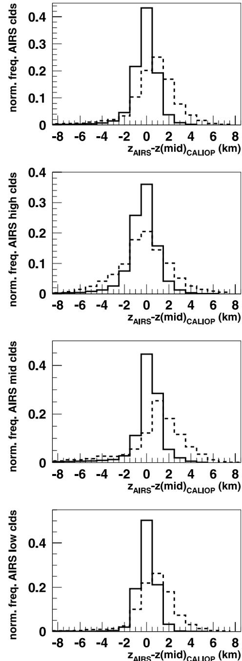
**Figure 7.** Normalized frequency distributions of the difference between AIRS  $z_{\text{cld}}$  and CALIPSO height of the apparent middle of the closest cloud layer with  $\tau_{\text{VIS}} > 0.1$  for all AIRS clouds and for AIRS high, midlevel, and low clouds, separately for clouds with  $\varepsilon_{\text{cld}} > 0.6$  (solid line) and clouds with  $\varepsilon_{\text{cld}} \leq 0.6$  (dashed line).
