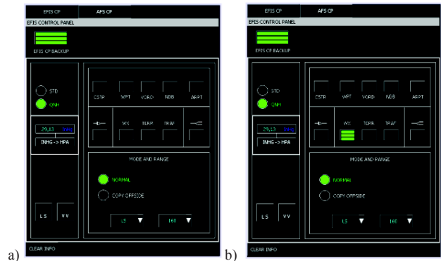
Figure 3. EFIS control panel (with (b) and without (a) the activation of the weather radar)
