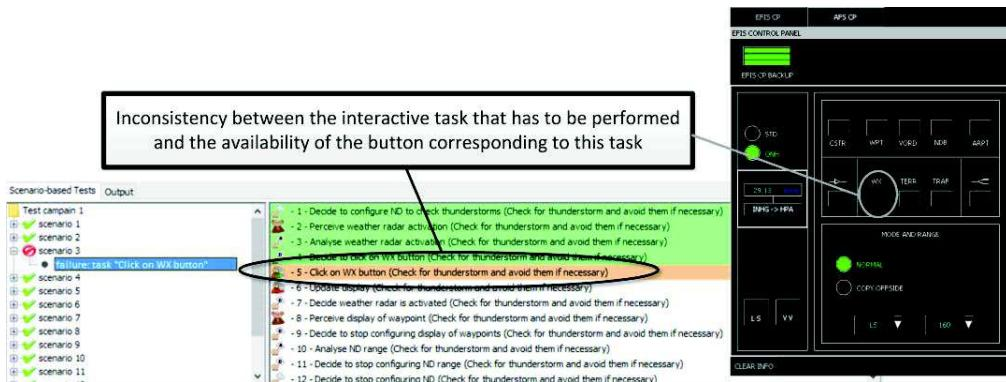
Figure 6. Results of the test campaign while the WX button has been disabled in the FCUS application
