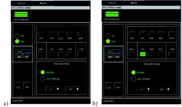
**Figure 3. EFIS control panel (with (b) and without (a) the activation of the weather radar)**
